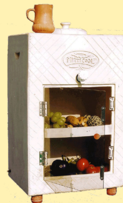
Mitticool: Water seeps from the upper chamber of the clay box, into the wall of the lower sections, where its evaporation keeps the stored food cold. (photo: © Mitticool)
